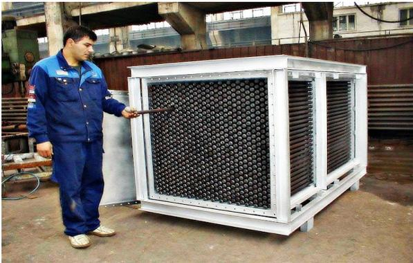
One of the unique features of the heat pipe heat exchanger is that there are no moving parts and therefore they require a minimal amount of maintenance. The operation of a heat pipe heat exchanger requires no external energy other than the thermal energy to be transferred.
